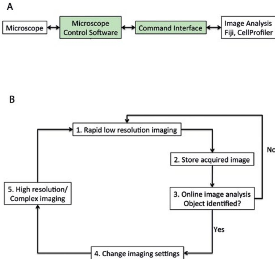
**Fig. 3:** Components and their communication in adaptive feedback microscopy (A) Components and their communication required for adaptive microscopy. The command interface enables communication between the microscope control software and image analysis packages and needs to be developed in a system specific manner. For feedback microscopy on a ZEISS LSM 780 a Visual Basic Macro as described earlier [5] is used as command interface. (B) Flow chart of a basic feedback microscopy experiment.
