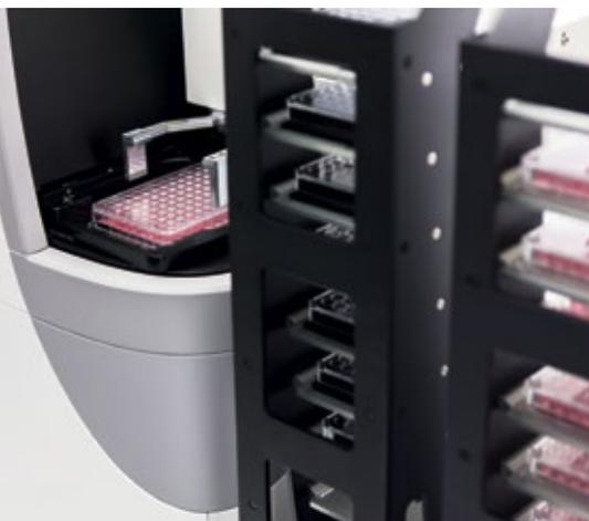
**Fig. 1:** Proper integration of robotic loaders into imaging systems can boost the degree of automation and thereby throughput. However, this is only one automation aspect and robotics must work seamlessly together with all other components of the system.
