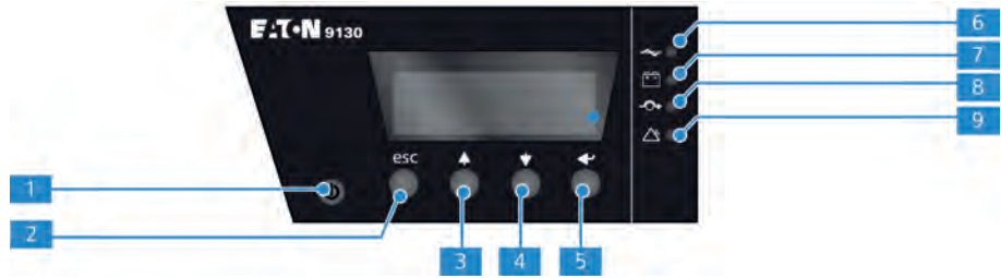
Fig. 2: Operator panel of the UPS
