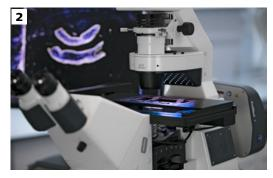
Without the need of manual sample positioning or focusing, an overview image for fast and convenient navigation is taken within seconds.
