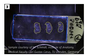
■ Intelligent routines automatically identify your sample carrier, regardless if you use a petri dish, a chamber slide, or a multiwell plate. Carrier properties are automatically transferred to the software, eliminating manual settings.
