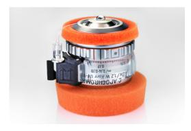
Create long-term live cell and multi-position experiments with automated water immersion.
