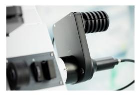
Excitation filter wheel for high speed multicolor imaging.
