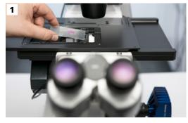
After you placed the sample on the loading position, the AI Sample Finder automatically moves it to the objective.
