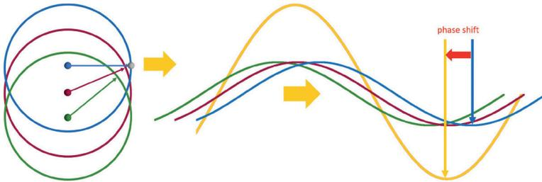
Schematic illustration of the slowing down of light in media with high optical density, exemplified by one electron (blue) and its two neighbors (red and green). While photons ‘jump’ from electron to electron at the full speed of light  $c$ , the resulting ‘light wave’ (orange) travels more slowly due to the consecutive phase delays. The refractive index  $n$  is a measure of the resulting slowing of light in media relative to a vacuum.
