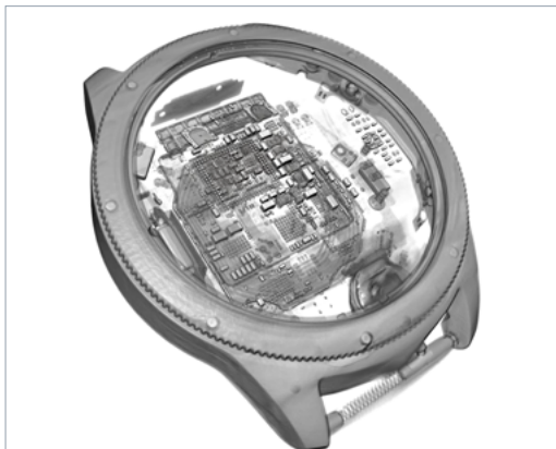
3D rendering image of smart watch imaged at 28 μm/vox. Image shows the entire watch assembly as well as the internal features such as motherboard and sound components.
