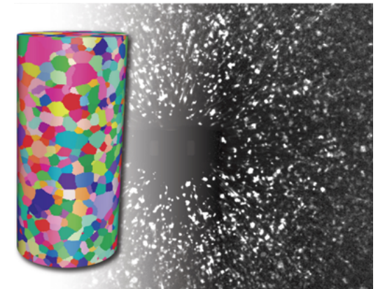
3D grain map of an armco iron sample with dimension of (diameter) 1.0 mm and (height) 3 mm. Sample scanned using helical phyllotaxis raster scheme. Sample courtesy of Prof. Burton R. Patterson, University of Florida, USA.
