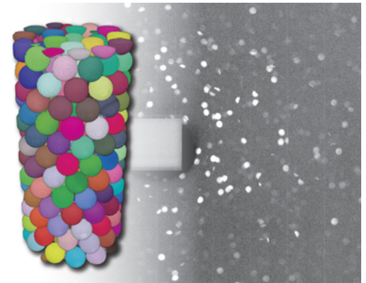
3D grain map of stacked sapphire spheres with individual sphere diameter of 0.2 mm. Sample scanned using helical phyllotaxis scheme.
