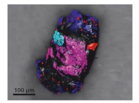
Correlation of the light microscope image with the EDS elemental analysis from the SEM
