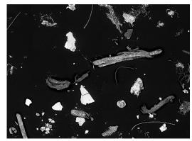
Gray-scale segmentation of particles by backscattered electron intensity
