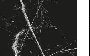
Particles and fibers from a construction site, including dust, wood and fibers from insulation materials. Asbestos particles identified by EDS indicated by colors in the right image.
