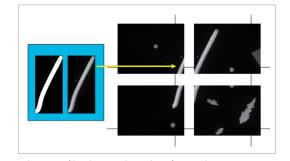
Schematic of border particle stitching feature showing composite stitched particle and constituents
