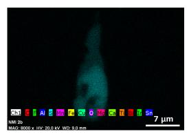
EDX measurement - sulfur content identified.
