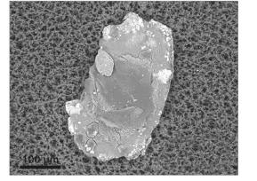
Backscattered electron microscopy image of the same particle
