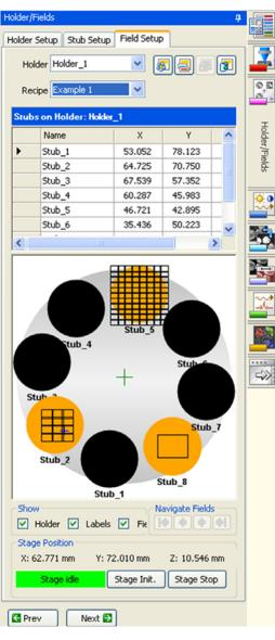
Sample holders include a single filter holder for individual particle investigations; and multi-sample holders for for up to nine filters or stubs, typically used for unattended measurements over hours or even days.
