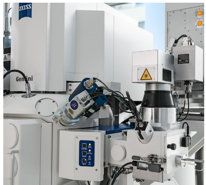
Figure 1. LaserFIB: ZEISS Crossbeam equipped with new femtosecond laser.
