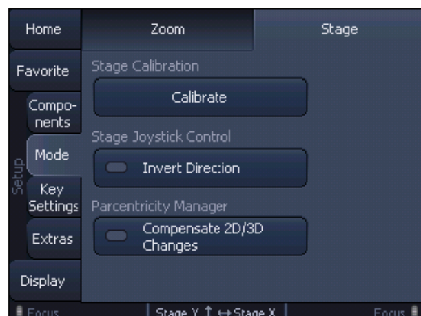
Fig. 10 Activating/deactivating the Parcentricity Manager
