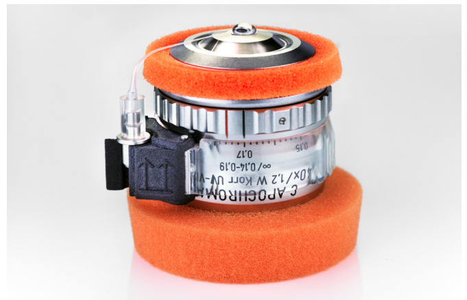
The Autoimmersion Module does not decrease working distance, nor does it block visibility or access to the correction collar.
