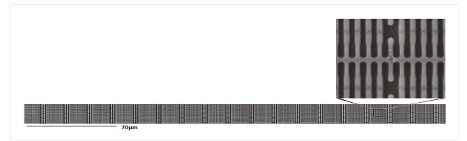
Bottom: Overview image of semiconductor device showing the capability of ZEISS Atlas 5 to also acquire non-square images. Top: Detail of semiconductor structure.
