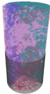
Mineralogic 3D combines X-ray microscopy with advanced machine learning to provide a true measurement of the sample with no obscured phases of interest
