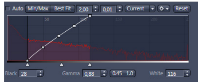
The same image displayed with a steep display curve – cutting away some of the dark and bright information – shows too much contrast.
