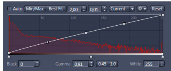
A nearly linear Gamma over the whole dynamic range delivers a rather dark display of this transmitted light image.
