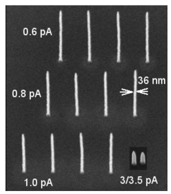
Figure 2 Dependence of pillar aspect ratio on applied beam current.
