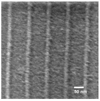
**Figure 5** *Platinum lines 15 nm wide, with a 100 nm pitch.*
