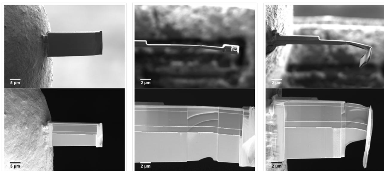
**Figure 3** Conventional FIB lamella preparation, side mount. SEM micrographs recorded with SE2 detector (top row) and Inlens SE detector (bottom row). The lamella is bending early during thinning. Further thinning is not possible.
