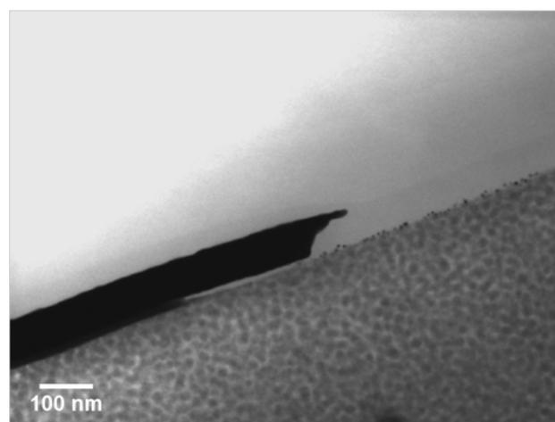
**Figure 6** 28 kV STEM brightfield image recorded from the  $X^2$  lamella in the ZEISS FIB-SEM.
