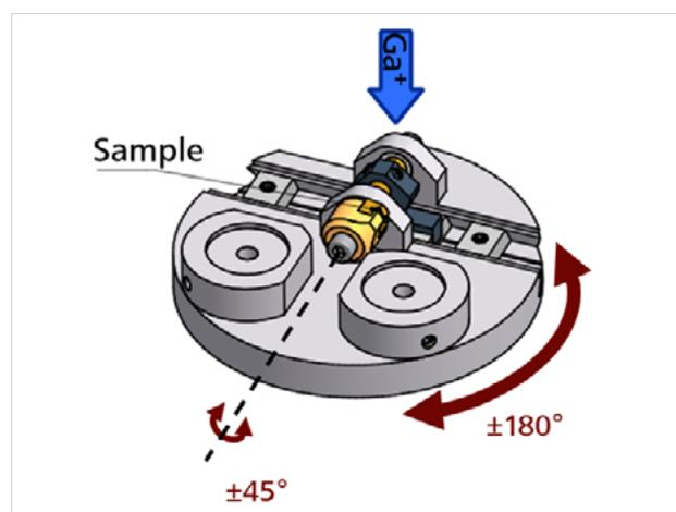
**Figure 2** X<sup>2</sup> sample holder. Rotation of the holder while the stage is tilted flips the TEM grid from the front side to the back side milling position.
