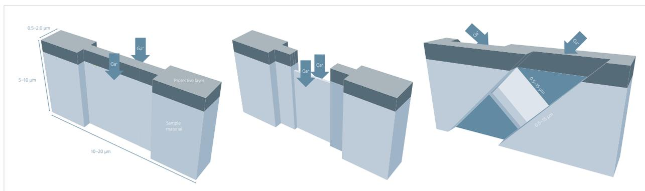
**Figure 1** Principle of conventional (left, center) and X<sup>2</sup> method (right) lamella thinning.
