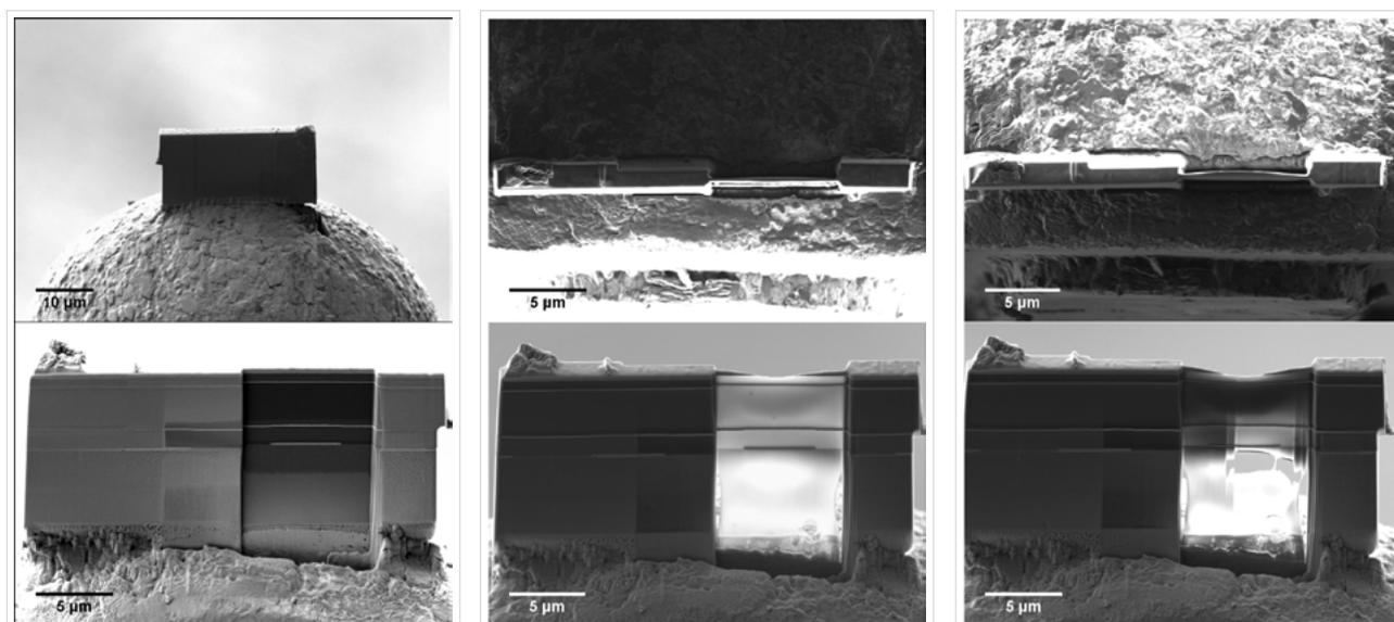
**Figure 4** Conventional FIB lamella preparation, bottom mount. SEM micrographs recorded with SE2 and Inlens SE detectors. Bending is reduced, but still present. When thinning further, this leads to uneven thickness and, eventually, to destruction of the lamella.
