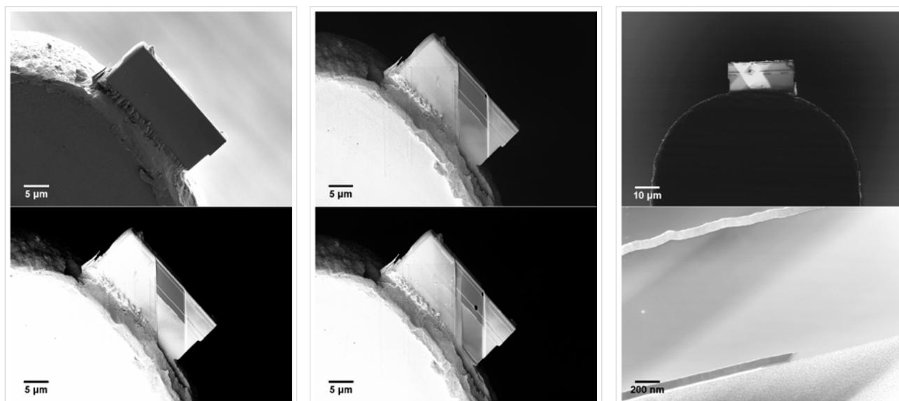
**Figure 5**  $X^2$  lamella preparation. SEM micrographs recorded with SE2, Inlens SE and (right column) STEM detectors. The lamella is thinned until a small hole appears, but no bending occurs.
