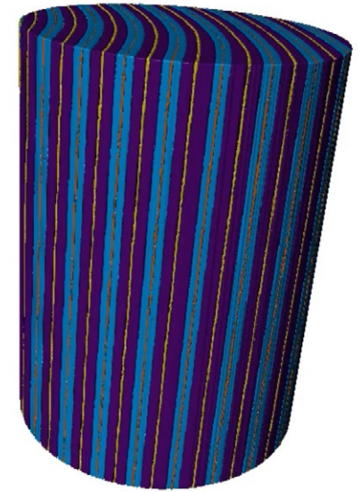
3D image of 21700 battery scanned by ZEISS Xradia 620 Versa
