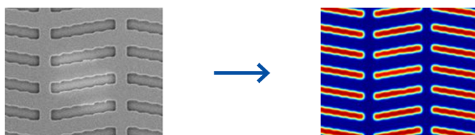
Photomask defect after repair: ZEISS MeRiT supports reliable mask repair and defect correction via gas-assisted electron beam lithography (on left). The aerial image captured with ZEISS AIMS (on right) enables the user to verify the quality of the repaired defect.
