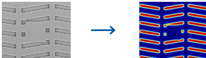
Photomask defect before repair: The SEM image captured with ZEISS MeRiT (on left) indicates the defect in the pattern, while the aerial image from ZEISS AIMS (on right) shows how this translates to wafer printing on the EUV photomask.
