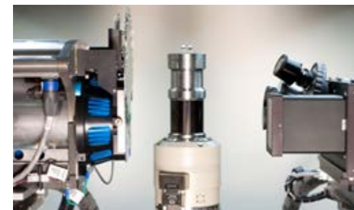
X-ray source (left), sample stage with tension/compression stage (center), and detector (right). Even with source to sample distances of several centimeters to accommodate in situ sample holders, voxel sizes below one micron can be achieved.
