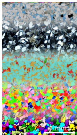
Composite multichannel acquisition of Berea Sandstone, showing Brightfield acquisition (top), crossed polarized (birefringent) acquisition, the result of phase segmentation (center), angular phase solution and identified crystal grains (bottom). Machine learning segmentation is used to classify pore (gold), quartz (light blue), Calcite (dark blue), Micas (red) and opaque minerals (green and yellow).
