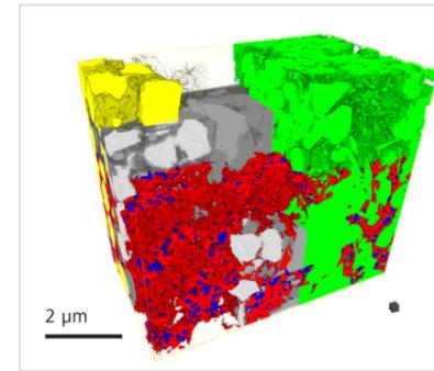
*Fracture in a sandstone created using integrated in situ uniaxial load cell. Imaged with ZEISS Xradia Versa 3D X-ray microscope.*
