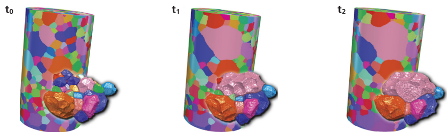
4D grain map of an Armco iron sample imaged at various annealing steps. t_0 : initial state; t_1 : after annealing at 880 °C for 8 hrs; t_2 : after annealing at 880 °C for 16 hrs. By imaging the sample at three temporal states, the abnormal grain growth of the top, pink-colored grain is captured. Courtesy of Prof. Burton R. Patterson, University of Florida, United States.
