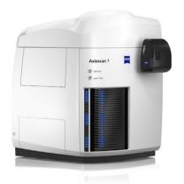
ZEISS Axioscan 7 Geo produces unique datasets for polarization microscopy with multiple light modes captured in multiple orientations. This enables digital thin sections to be viewed within a virtual petrographic microscope or interrogated for pixel or grain scale information.
