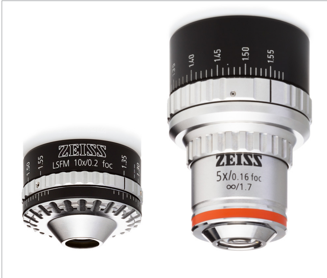
Figure 3 ZEISS Lightsheet 7 illumination objective 10x/0.2 foc and detection optics 5x/0.16 foc. Both feature a new focus adjustment ring to tune the illumination (light sheet) and detection focus to the chosen medium.
