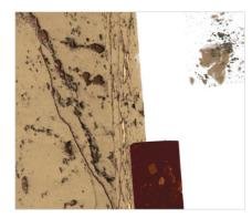
Volume segmentation showing interior location of gold in core sample. ZEISS Xradia Versa X-ray microscope
