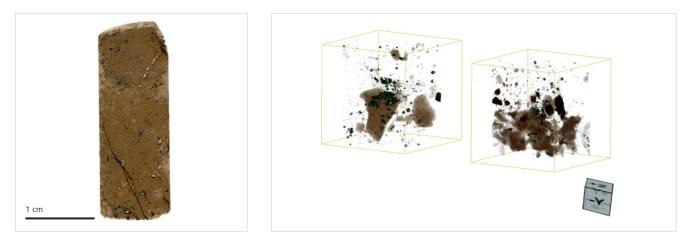
"Scout" the entire drill core (segmented to show the different mineral groups of silicates and sulphides) and then "Zoom" to show the gold mineralization particles using non-destructive 3D X-ray microscopy.
