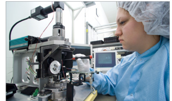
From around 7,000 reference points, the zoom body adjustment device calculates the zoom control curve.
