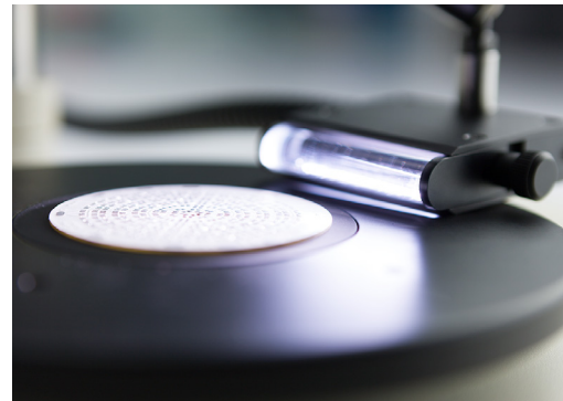
Line light S provides a homogeneous carpet of grazing light. Use it to contrast surface structures of large flat specimens with strong shadows.
