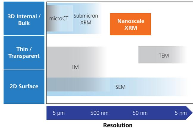
Figure 1. Approximate imaging resolution for common in situ mechanical testing methods, categorized by sample thickness and transparency. The in situ Xradia Ultra Load Stage uniquely fills a gap between single nanometer resolution SEM/TEM methods that are restricted to surface imaging or extremely thin samples, and micron/submicron-scale tomography.
