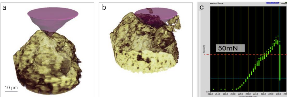
Figure 3. Nanoindentation of dentin. (a) 3D rendering of dentin sample before cracking. The indenter tip is visible above the sample. (b) 3D rendering of the same sample after the indenter tip has been driven into the sample and a piece of dentin has fractured off. (c) Force-displacement curve. The fracture event is clearly visible. Courtesy The University of Manchester.
