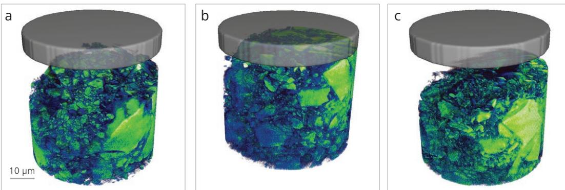
Figure 2. Compressive loading of a porous elastomer. (a) Uncompressed, (b) Compressed, (c) Decompressed
