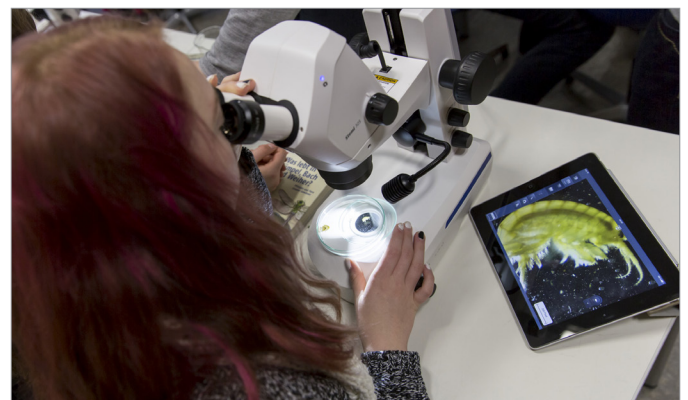
Figure 11 Students working with a Stemi 305 cam. The microscopic image is visualized using Labscope on an iPad.
