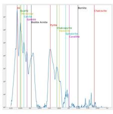
Mineral classifications based on attenuation measurements
