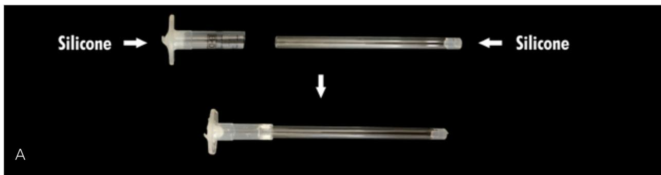
**Figure 1** Illustration of the steps to seal the Simax tube that will contain the non-compatible chemicals. The cut barrel of 1 ml syringe is sealed with silicone as well as the Simax tube. Then, the sample cleared with ARIM is inserted in the tube and covered with fresh ARIM. Finally, both parts are mounted together.
