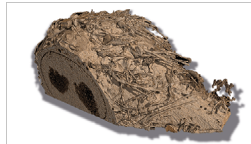
Individual cells grown in a cell culture, chemically-fixed and resin-embedded. Acquired using Atlas 5 3D Tomography at a voxel size of 5 × 5 × 8 nm over a total length of 16 μm. Usage of the EsB detector allows to image ultrastructural details without charging artifacts typical for resin-embedded samples. The video (left) shows a fly-through of 1400 slices. The 3D visualization (right) was done using ORS Dragonfly Pro software. Courtesy of: A. Steyer & Y. Schwab, EMBL Heidelberg, Germany. (Field of view 44 μm × 28 μm).
