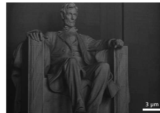
A FIB grayscale rendering of the Lincoln Memorial is patterned into silicon with the FIB beam. An unmodified photograph was used as the data source. Patterning time: 10 minutes.
