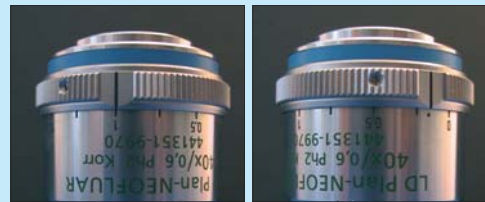
Regular glass slide (1 mm thick) => 1, thin slide (0.17 mm thick) => dot, DuplexDish => between dot and 0.
