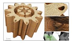
3D scan of Al component produced by additive manufacturing and, inset, internal porosity imaged via X-ray microscopy
