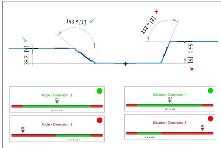
Tolerance limits can be set on measurement parameters and surface roughness measurements. Comparison to CAD files as well.
