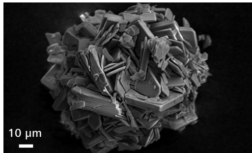
C2D imaging with drastically reduced charging effect (Sample: Lanthanum carbonate, a phosphate binder used as an oral therapeutic agent for dialysis patients.).
