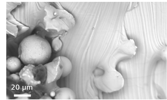
Surface of titanium alloy (Ti-6Al-4V) additively manufactured using selective laser melting, showing fully melted regions alongside unmelted Ti-6Al-4V particles and other material. Imaged with BSE detector on EVO 15. Sample provided by TWI Ltd.
