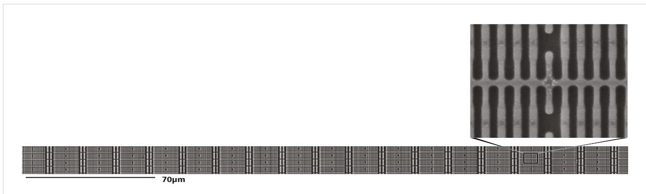
Bottom: Overview image of semiconductor device showing the capability of ZEISS Atlas 5 to also acquire non-square images.
