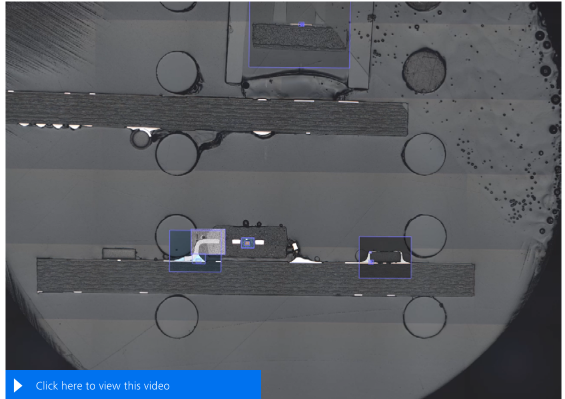
Multi-modal investigation of an electronics part, connecting images from light microscopy, SEM and analytical data in EDS maps. View of the GUI of the correlative workspace of a ZEN Connect project with aligned data. Sample: Electronics part, embedded and mechanically polished cross-section. Sample: courtesy of Aalen University, Materials Research Institute, Aalen, Germany.
