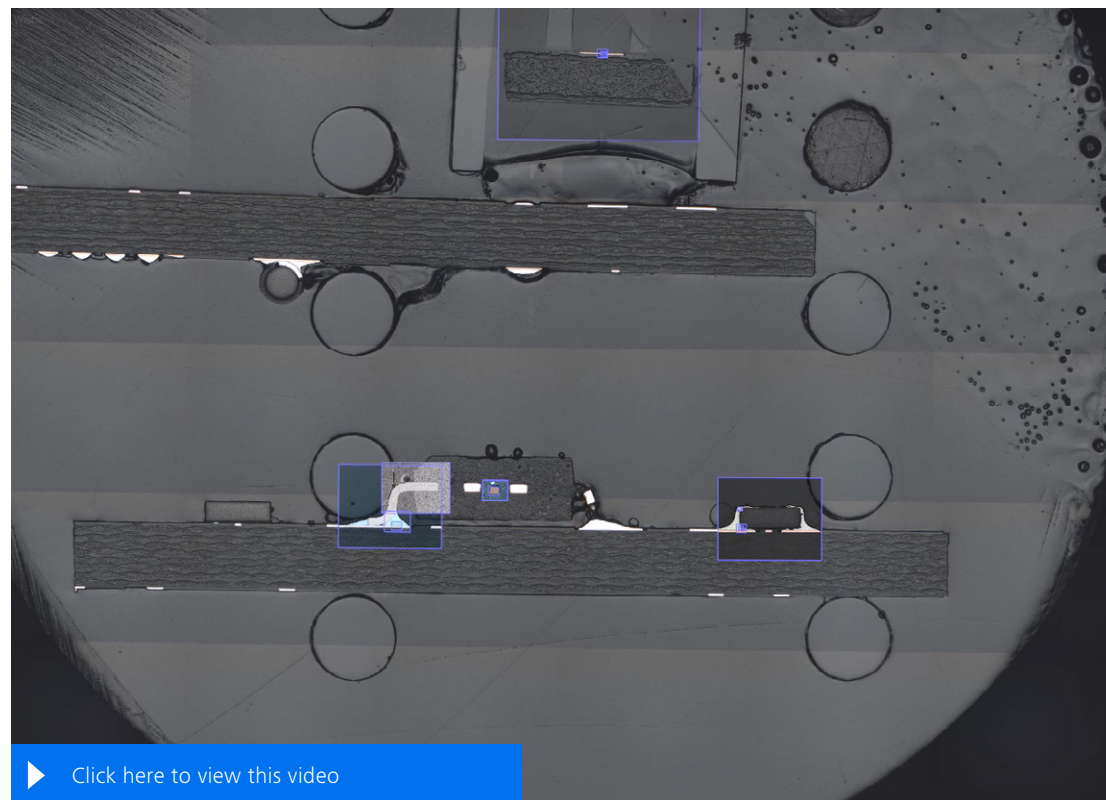
Multi-modal investigation of an electronics part, connecting images from light microscopy, SEM and analytical data in EDS maps. View of the GUI of the correlative workspace of a ZEN Connect project with aligned data. Sample: Electronics part, embedded and mechanically polished cross-section. Sample: courtesy of Aalen University, Materials Research Institute, Aalen, Germany.
