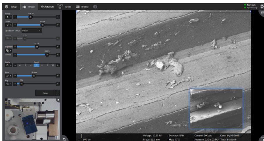
Figure 1 ZEISS SmartSEM Touch control system. Example shown is routine simultaneous dual-channel imaging of a coated screw thread using secondary electron imaging and backscattered electron imaging. All parameters are easily controllable by touch, mouse or ZEISS control panel.
