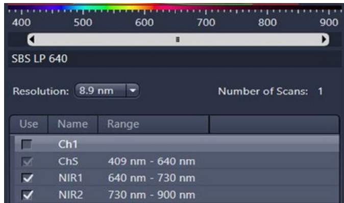
Figure 9 Spectral detection GUI, integrating several detector types which can be used with LSM Plus.
