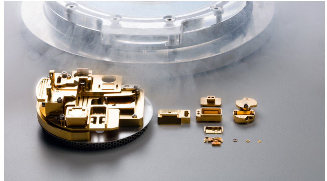
TEM prep slusher of the Quorum Prepdek ® workstation with ZEISS Perspex lid; components of the ZEISS Cryo Accessory Kit
