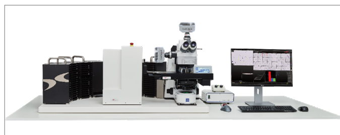
Figure 5 A complete installation with the Metafer software. The hardware consists of an Axio Imager Z2 microscope, a motorized scanning stage, and MetaSystems' CoolCube4 cameras. The optional SlideFeeder x80 slide frame feeder is shown on the left.
