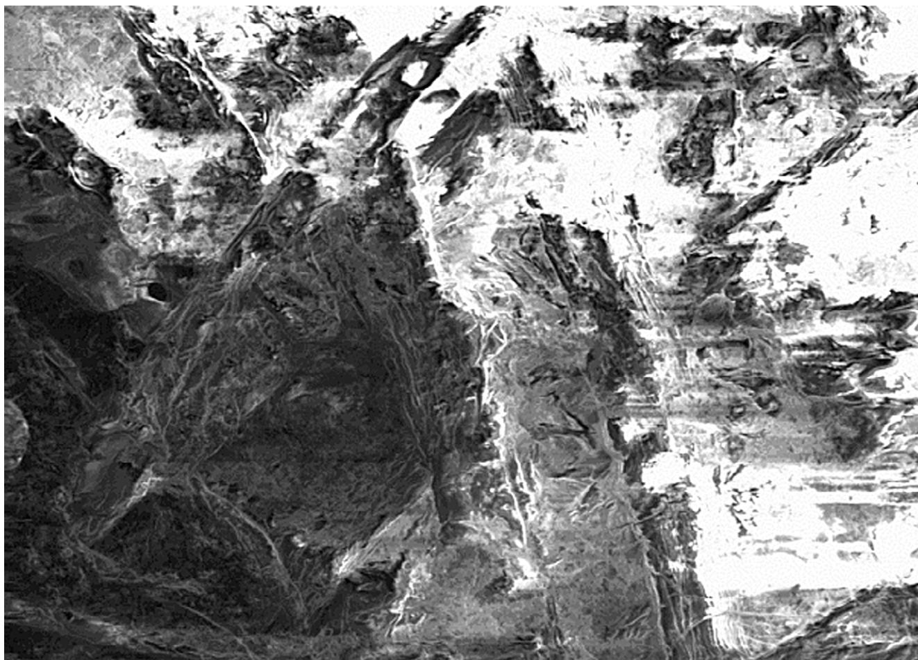
Figure 2 Secondary electron image of the internal structure of copy paper obtained in high vacuum and without prior preparation. The analysis conditions are 3 kV, Everhart-Thornley SE detector. The "charging" artefacts include the white horizontally streaked areas to the top and right of the field together with a distortion of the image. The horizontal field of view is 140 \mu\text{m} .
