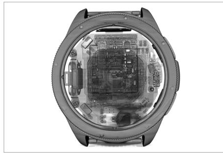
3D microCT scan of smartwatch (left) and smartwatch motherboard showing SMT components and BGA bump array (right), 2.85 \mu\text{m}/\text{voxel} .
