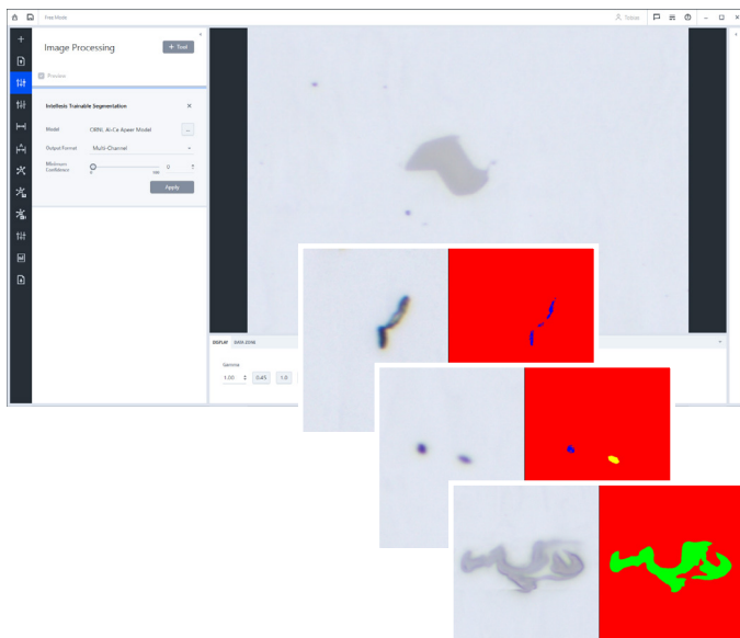
Figure 7: Segmentation of the different objects – blue: Zr-In inclusion; yellow: pore; green: oxide
