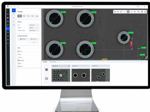
Metrological inspections and analyses of microscopy data are performed automatically by the ZEISS ZAPHIRE software.
