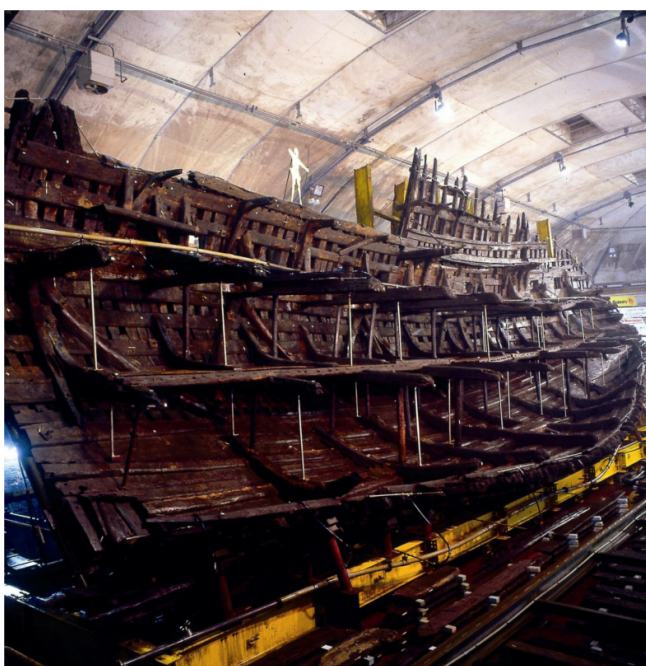
Figure 1 The remains of the Mary Rose's hull. All deck levels can be made out clearly, including the minor remnants of the sterncastle deck.
