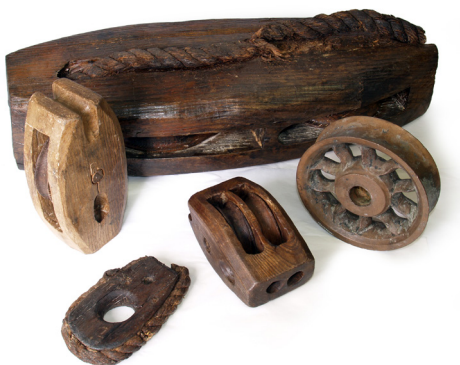
Figure 3 A small selection of the many rigging blocks raised from the Mary Rose.
