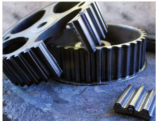
Figure 3 Example of failed component: cracked gear from an engine timing component.
