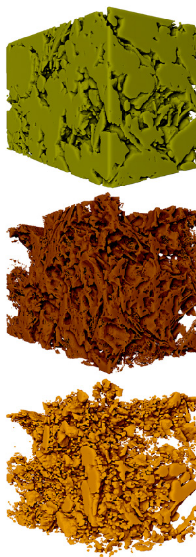
Figure 3 Digital rock model of Marcellus Shale Sample-2 – pores (yellow), organic matter (brown), mineral matter (green).
