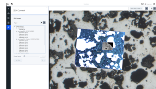
Perform correlative or multi-modal microscopy. The user interface of ZEN core is specifically tailored to complex, sample-centric experimental setups. All images are visualized in what's known as a correlative workspace; multi-modal, multi-scale data can be aligned and put into context in a single ZEN Connect project – for example, correlate light microscope with SEM images and EDS maps.
