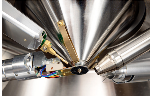
A look inside the chamber with the annular BSE detector (aBSD) mounted under the pole piece of the objective lens enabling imaging in variable pressure (NanoVP lite mode).
