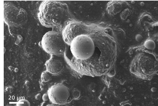
Aluminum chlorohydrate from an aerosol antiperspirant obtained at 7 kV and 25 Pa chamber pressure with VPSE.
