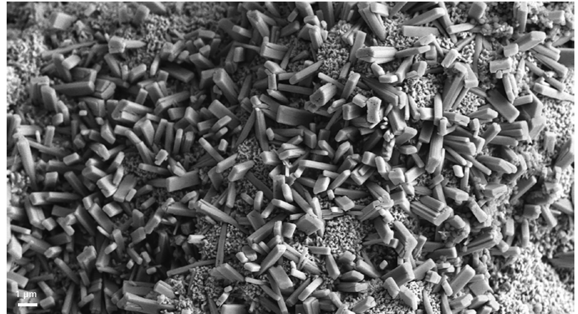
This image of zinc oxide dendrites aids detection of morphological changes in the electrodes of energy storage systems. Secondary electron imaging using the ETSE detector on Sigma.
