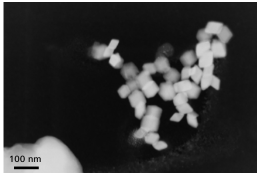
25 – 50 nm iron oxide particles imaged with the aSTEM detector in darkfield mode at 20 kV.
